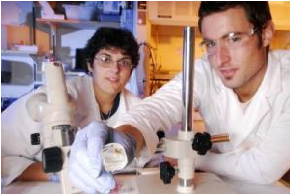
Georgia Tech research technician Kellie Templeman (left) and former graduate student Tim Petrie display a piece of titanium coated with a bio-inspired polymer that enhances bone formation around the metal after implantation. (Credit: Georgia Tech Photo: Gary Meek)
